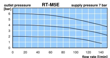
\*1 for compressed air: 7 bar supply pressure, 6 bar outlet pressure and 1 bar pressure drop
