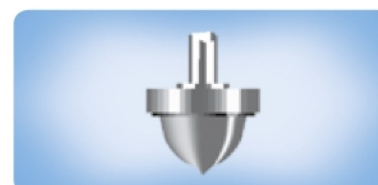
parabolic piston enables stroke-proportional K v value change
