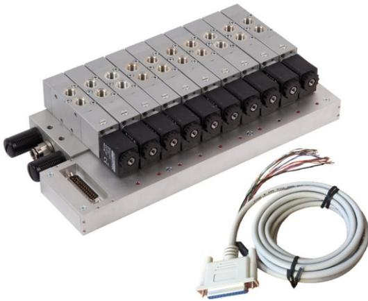
This system allows the installation of a series of 1/8 solenoid valves with different functions: 5/2 monostable 5/2 bistable and 5/3, through a printed circuit board inserted in an aluminum shell with a female connection SUB-D 25 pin; this avoids the wiring of each valve.
