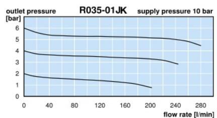
\*1 for R364-J at 8 bar supply pressure or R035-J at 10 bar supply pressure, 6 bar outlet pressure and 1 bar pressure drop
