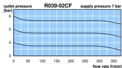
\*1 at 7 bar supply pressure, 6 bar outlet pressure and 1 bar pressure drop, for water: supply pressure 2 bar above outlet pressure
