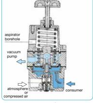
cross-section connection for downstream regulation
