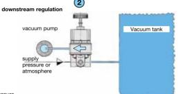
A strainer is provided on the pressure side or atmospheric, an additional filter is recommended.
