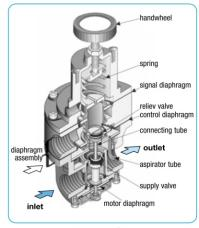
cross section connection for downstream regulation
